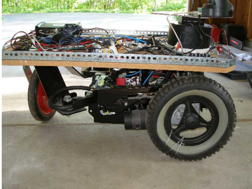
Figure 1: Our modified wheelchair base during the build process.
