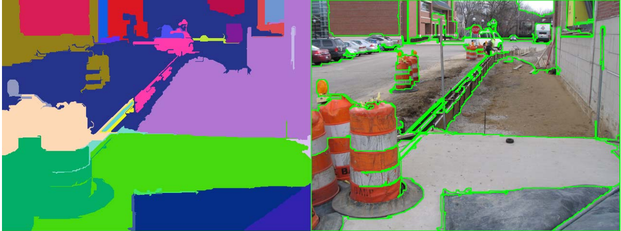
Figure 7: A construction scene with obstacles that has been segmented out using the graph-based image segmentation code.
