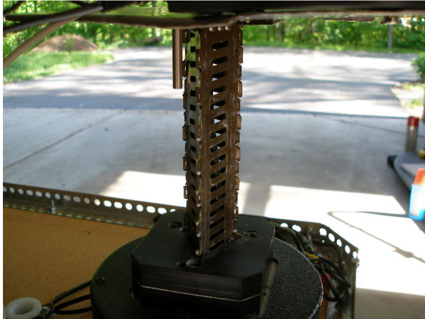
Figure 4: The SAM, Situational Awareness Mast, which we are using to mount our camera and GPS receiver on.
